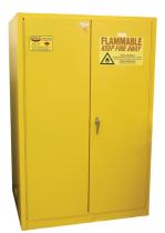
Approved cabinets may contain up to 60 gallons of class I flammables and/or class II combustibles, or up to 120 gallons of class III combustibles.
