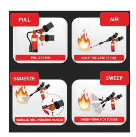
Fire extinguishers should be inspected monthly to confirm adequate pressure (gauge in the green zone), the pin is in place, and it is stored off the floor in a marked location. Initial and date the monthly inspection of each extinguisher on an attached tag. If an extinguisher has been used, never return it to its original location until it has been refilled and pressurized, or replaced with a new extinguisher.
