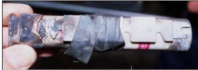
A melted fuse was repaired by taping a renewable fuse link on the outside.
