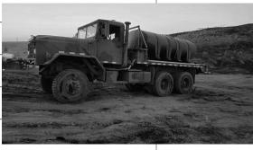
Logan Padget of Grass Valley Oregon started with a 1985 M923 miliary truck and built "The General." This six wheel drive truck has a load capacity of five tons, carries 1650 gallons of water, and pumps at 120 psi through 100 feet of hose or the water cannon on the front bumper that is controlled from inside the cab.
