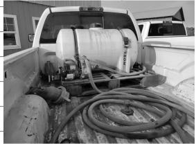
Assembled on the farm, this basic pump and extra tank in the back of a pickup. This is mounted on a pallet so it can be easily loaded into the truck when needed.
