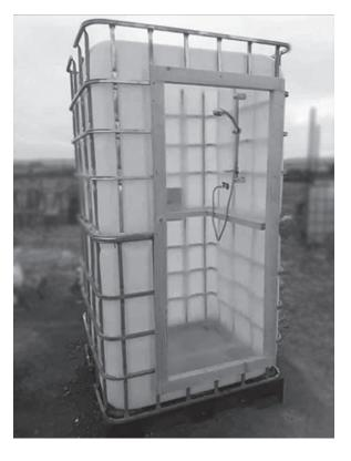
Two plastic totes, a shower head, tubing, some wire, and a few trim boards can produce a field shower. Consider using an elevated third tote filled with water and naturally warmed in the sun for a gravity fed warm water source.
