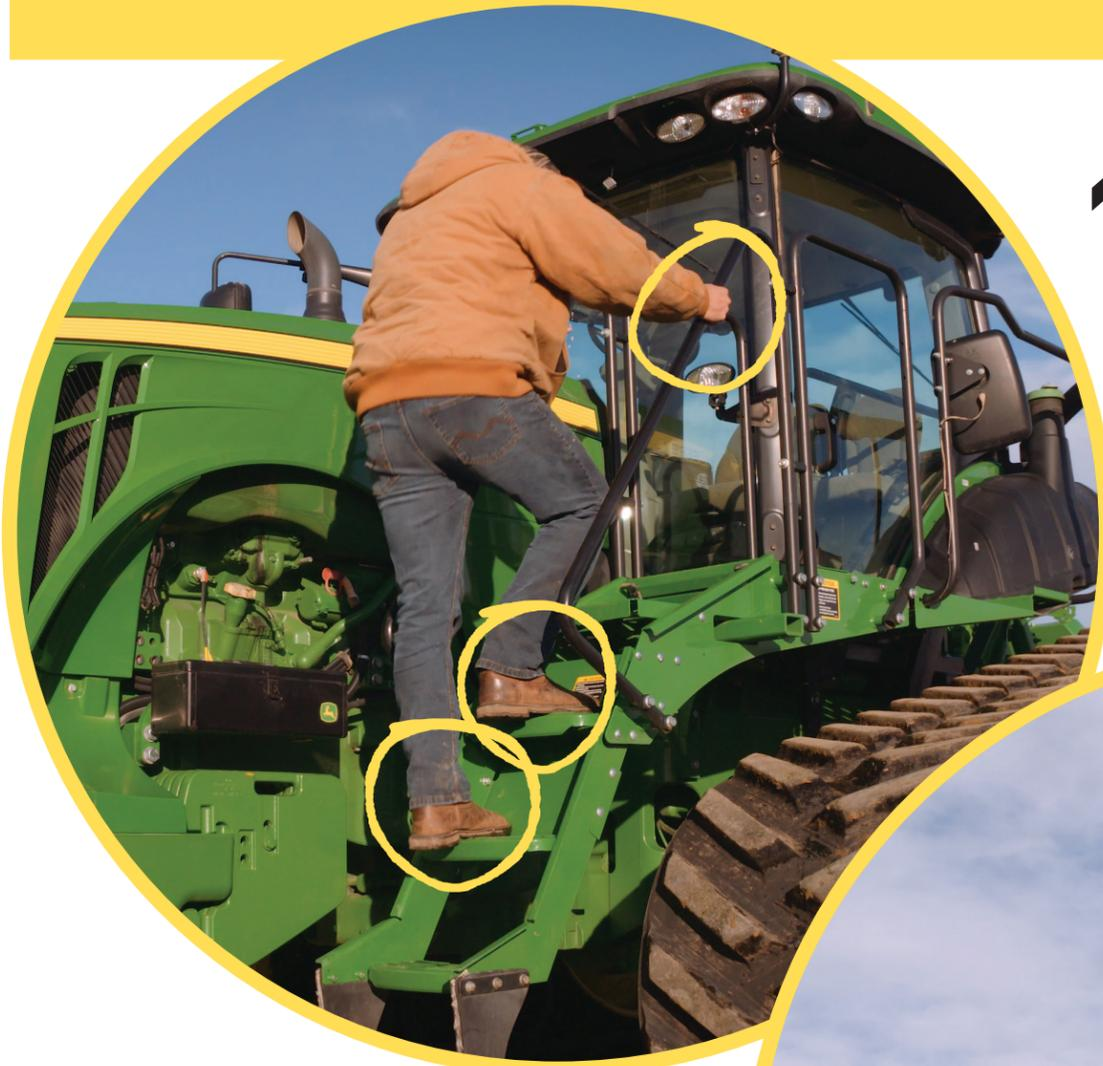
**1** Use secure points of contact (steps, running boards, hand- and foot-holds).
