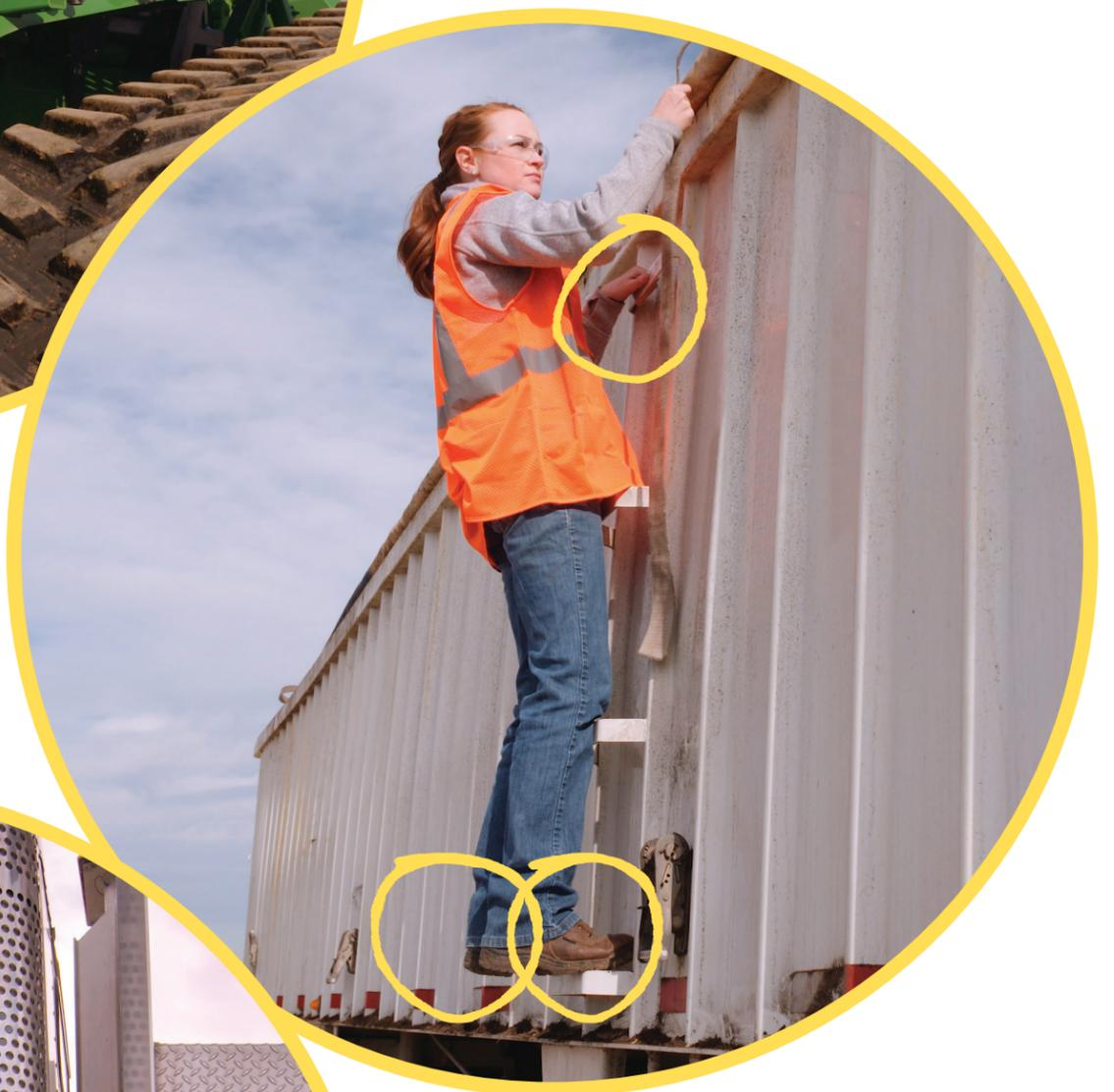
**3** Break contact only when you are safely on the ground or in the cab.
