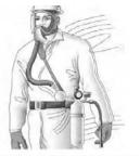
Full Facepiece Supplied-Air Respirator (SAR) with an auxiliary Escape Bottle APF=1,000 APF=10,000 (if used in "escape" mode) Needs to be fit tested
